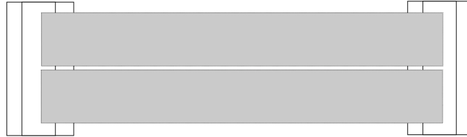
Figure 9 Top view of one middle segment of boardwalk
